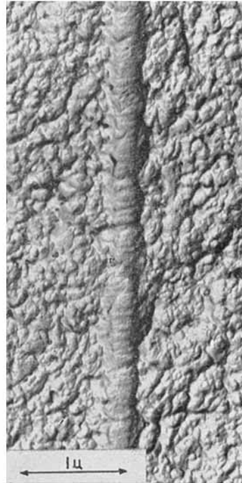
Fig. 5. Impact-fractured poly(methyl methacrylate). Electron micrograph of the cross section of a craze.
