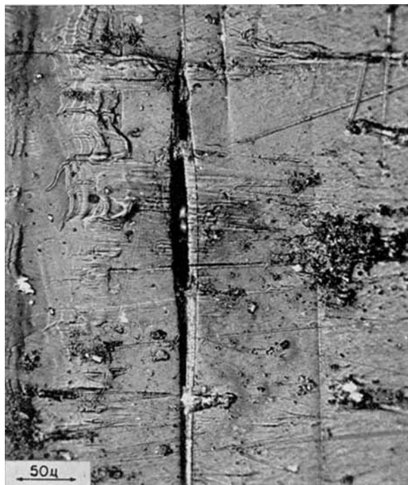
Fig. 1. Optical micrograph of a partially broken craze on the surface of a polycarbonate tensile test bar.
