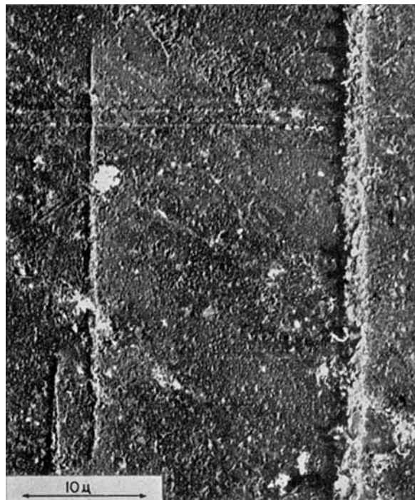
Fig. 2. Electron micrograph of a negative replica showing a small narrow craze and a portion of a wide craze. Same sample as Figure 1.
